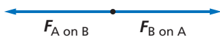
■ Figure 4-11 When you exert a force on your friend to push him forward, he exerts an equal and opposite force on you, which causes you to move backwards.
