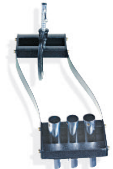
■ Figure 7-13 An inertial balance allows you to calculate the inertial mass of an object from the period ( T ) of the back-and-forth motion of the object. Calibration masses, such as the cylindrical ones shown here, are used to create a graph of T^2 versus the mass. The period of the unknown mass is then measured, and the inertial mass is determined from the calibration graph.
