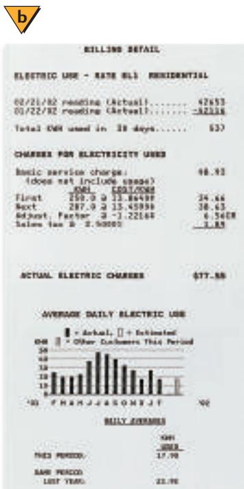
■ Figure 22-11 Watt-hour meters measure the amount of electric energy used by a consumer (a). Meter readings then are used in calculating the cost of energy (b).
