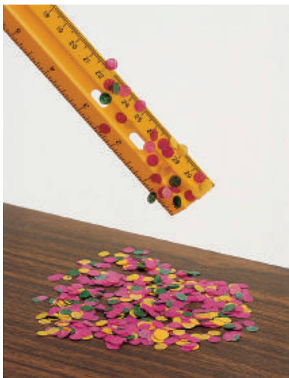
■ Figure 20-1 Rubbing a plastic ruler with wool produces a new force of attraction between the ruler and bits of paper. When the ruler is brought close to bits of paper, the attractive electric force accelerates the paper bits upward against the force of gravity.
