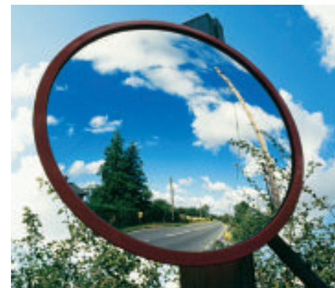
■ Figure 17-15 Convex mirrors produce images that are smaller than the objects. This increases the field of view for observers.
