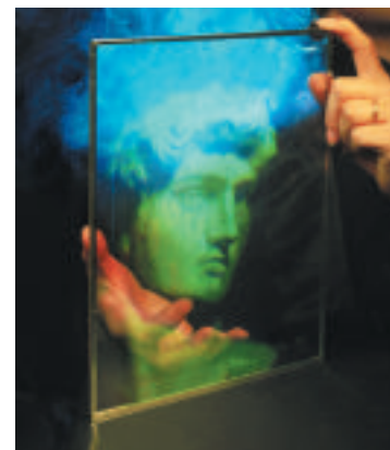
■ Figure 28-20 A hologram is formed when interference of two laser beams records both the intensity and phase of light from the object on film.
