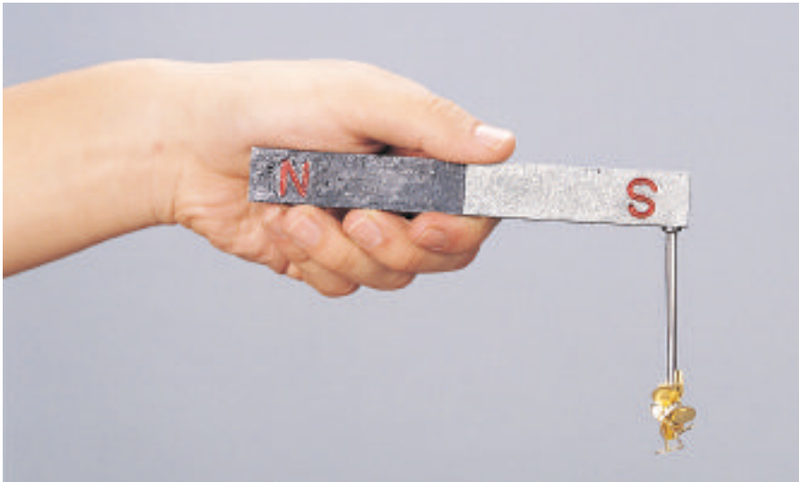
■ Figure 24-3 A common nail is attracted to a magnet. In the process, the nail itself becomes magnetized. Here you can see when a magnet is touching the nail, the nail is able to attract other metal objects. However, if you separate the magnet from the nail, some of the objects will drop off because the nail will have lost some of its magnetism.
