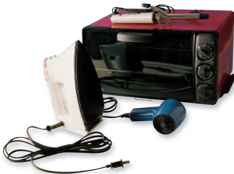
■ Figure 22-9 These appliances are designed to change electric energy into thermal energy.
