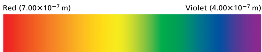
■ Figure 16-11 The spectrum of light ranges from the long, red wavelength to the short, violet wavelength.
