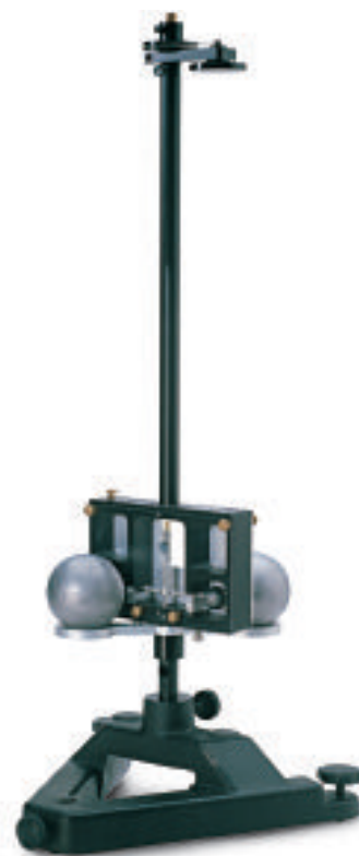
■ Figure 7-6 Modern Cavendish balances are used to measure the gravitational forces between two objects.
