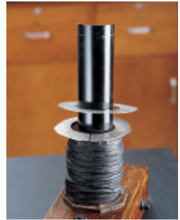
■ Figure 25-11 Current is induced in the continuous metal ring, while there is no current in the cut ring.
