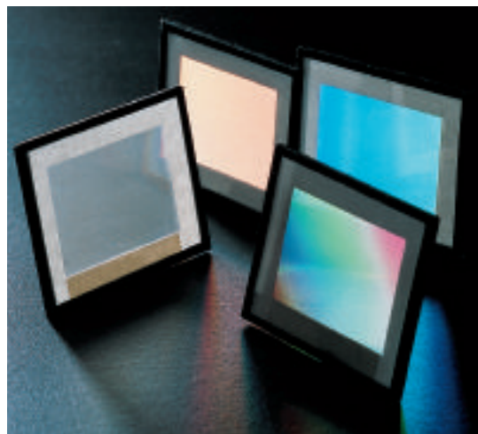
■ Figure 19-11 Diffraction gratings are used to create diffraction patterns for the analysis of light sources.
