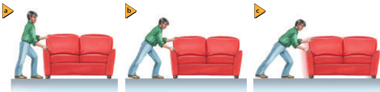
■ Figure 5-8 There is a limit to the ability of the static friction force to match the applied force.
