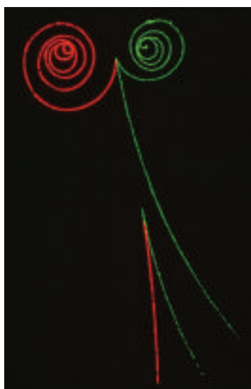
■ Figure 30-18 When a particle is produced, its corresponding antimatter particle is also produced. Here, a gamma ray decays into an electron-positron pair.
