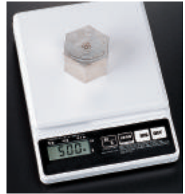
■ Figure 1-12 Accuracy is checked by measuring a known value.
